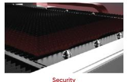
Multi-Directional design with ball bearings for easy edge feeding to avoid scratching the paper surface.
